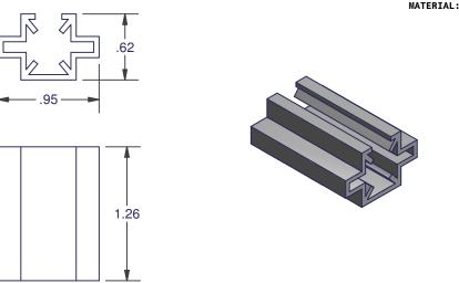
INSTALL IN NON-KEYED CYLINDER CAVITY OF EXTERIOR PULL FOR ADDED SECURITY.
